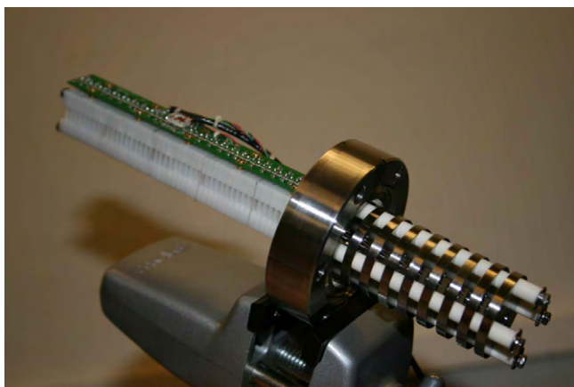
Fig. 2. Ion focusing assembly. The ion funnel spacers and the printed circuit board are shown on the left and the Einzel lenses and ceramic spacers are shown on the right. Both ion focusing elements are mounted to a modified, double-sided 2-3/4 in. Conflat flange.
